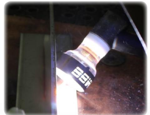
Using the included o-ring the Furick glass gas nozzles are attached to the welding torch:
