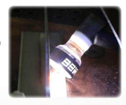
Using the included o-ring the Furick glass gas nozzles are attached to the welding torch:
