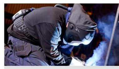
**Extended protection:** A flame-resistant headcover (used in this application) and ear/neck protection are available as accessories to all Speedglas 9100 series welding helmets.
